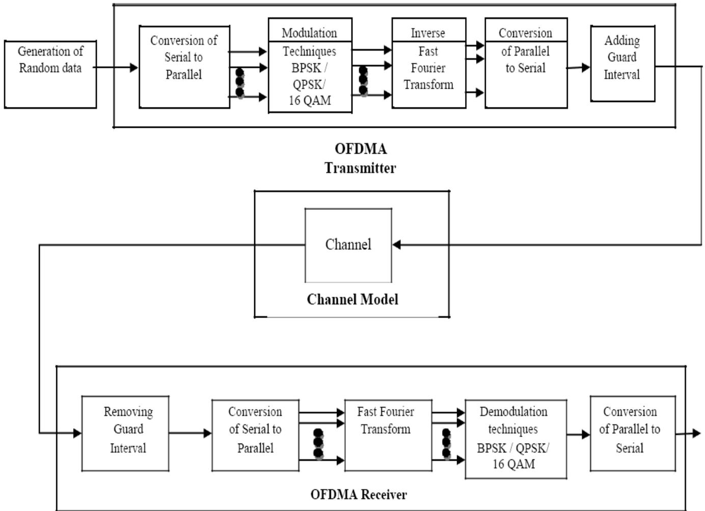
**Figure 1:** Transmitter and Receiver Block Diagram of OFDMA
