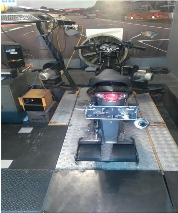
**Figure 5.** Engine Test Placement above Dynamometer
