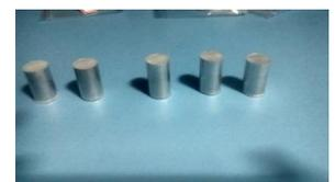
Figure 8. Specimens after sintering
