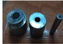
Figure 5. Hardened steel die and plunger for compression
