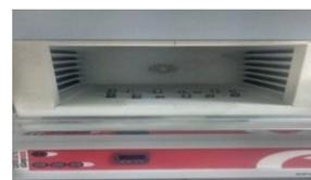
Figure 7. Muffle furnace for sintering
