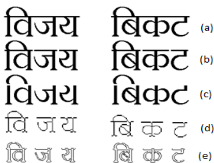
Figure 3. Preprocessing of Images (a) Original Image (b) Segmented Image (c) Elimination of Shirorekha (d) Thinned Image (e) Image Edging
