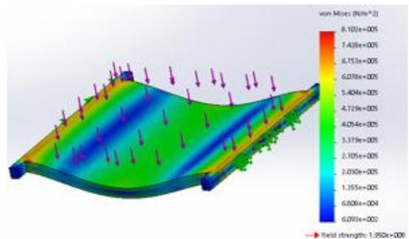
**Figure 3.** Von Mises stress of Main Base
