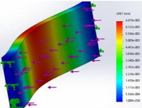
**Figure 8.** Displacement of X Axis Base
