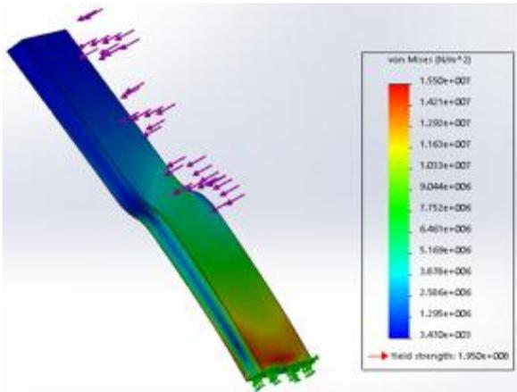
**Figure 5.** Von Mises Stress of Stand/ Column Y Load Direction
