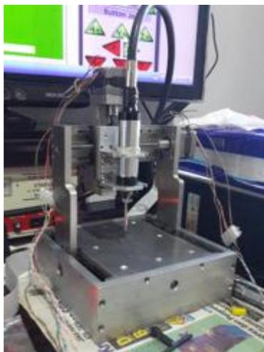
**Figure 12.** Portable CNC Milling Machine PM1035
