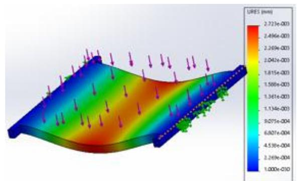
**Figure 4.** Displacement of Main Base
