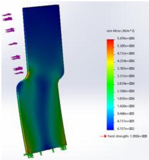
**Figure 6.** Von Mises Stress of Stand/ Column X Load Direction
