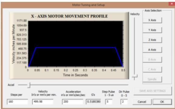
Figure 18. Motor Tuning Display
