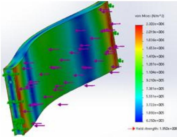
**Figure 7.** Von Mises Stress of X Axis Base
