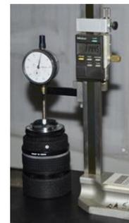
Figure 5: Measurement of height from window glass to front face of lens assembly with the use of dial gauge indicator
