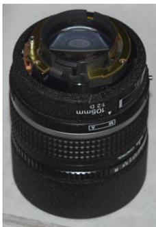
**Figure 8:** Removal of aperture adjustment ring
