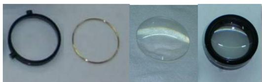
Figure 15: Removal of Lens 5
