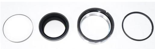
**Figure 12:** Removal of Lens 1 and distance measurement and Removal of Lens 2 and 3.
