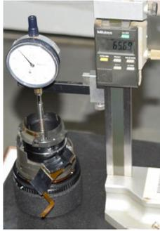
**Figure 11:** Removal of Lens Group (4, 5 and 6) and height measurement of aperture stop
