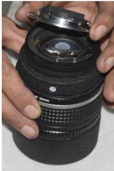
**Figure 7:** Removal of Rear Glass Window in its mount.
