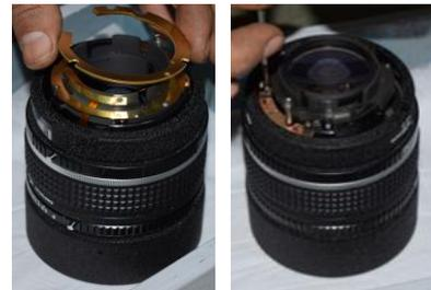
**Figure 10:** Removal of focusing ring
