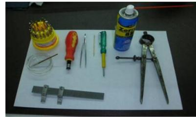
Figure 4: Tools required for dismantling of lens assembly
