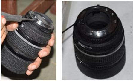
**Figure 6:** Application of solvent on the screws
