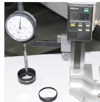
**Figure 14:** Removal of Lens 6 and measurement of separation distance from consecutive lens elements.
