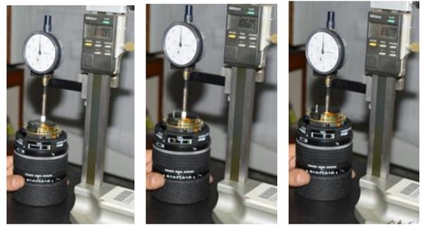
**Figure 9:** Height measurement of lens group at various focusing distance
