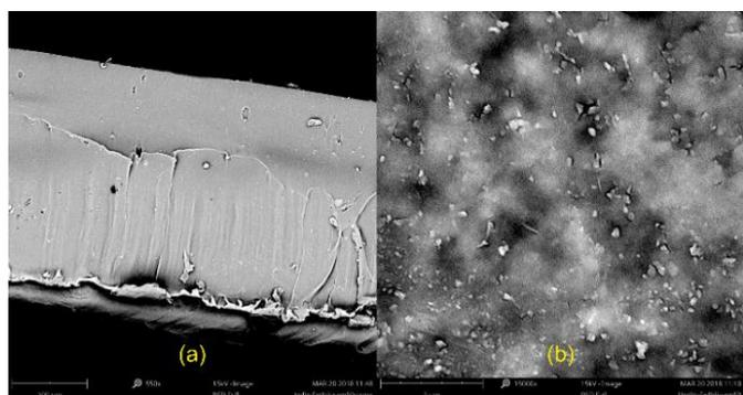
**Figure 7.** SEM Image of SAM 50 PEDOT:PSS Film (a) Cross Section (b) Surface Area
