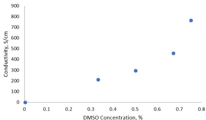
**Figure 8.** SAM PEDOT:PSS Films Electrical Conductivity
