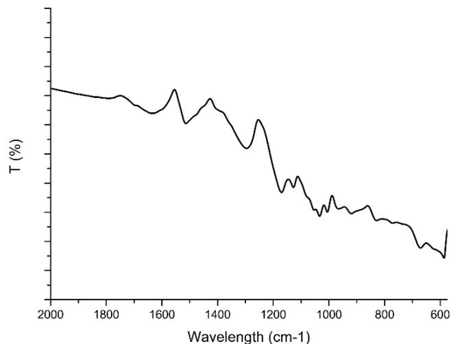
**Figure 4.** IR Spectra of Pristine PEDOT:PSS Flexible Film
