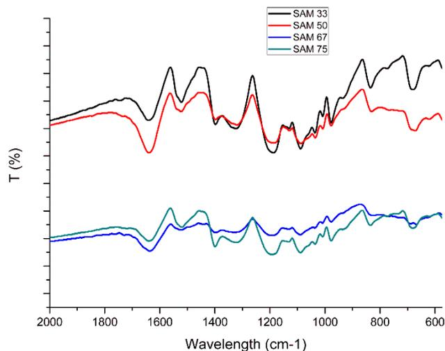
**Figure 5.** IR Spectra of SAM PEDOT:PSS Flexible Films
