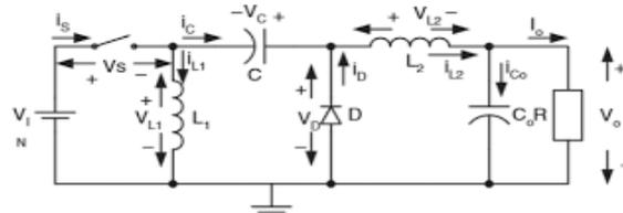
Figure 2. Elementary Luo Converter Circuit
