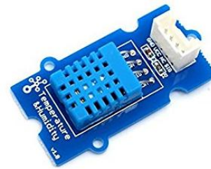
Figure 2. Temperature and Humidity Sensor
