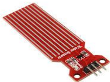
Figure 4. Water level Sensor
