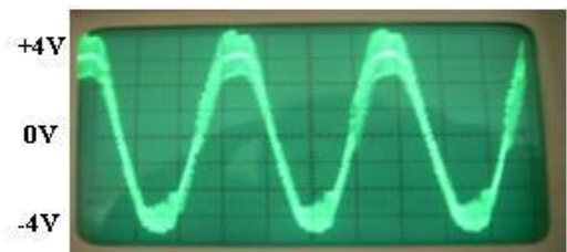
Figure 5.3. The compensation Voltage waveform after switching ON of the DVR when the DVR is ON.
