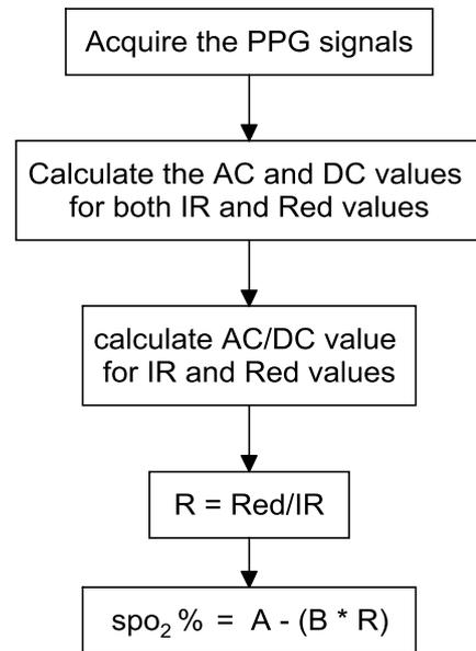
**Figure 2.** Program Flow for SpO<sub>2</sub> Measurement
