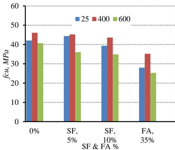
**Figure 2:** The effect of cement replacement by SF and FA on  $f_{cu}$  at different temperature.
