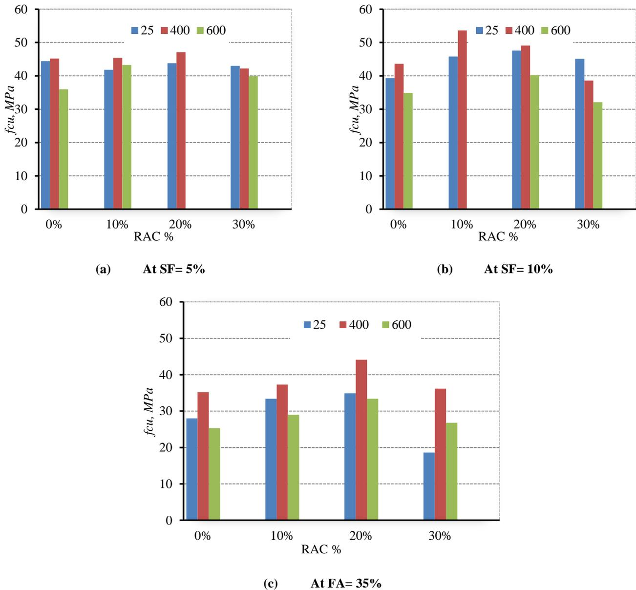
**Figure 4:** The Effect of the combination of RAC, SF and FA replacement on  $f_{cu}$  at different temperatures.
