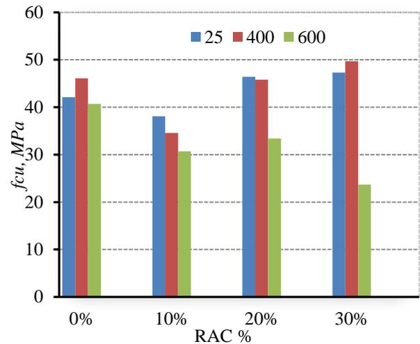
**Figure 3:** The effect of NA replacement by RAC on  $f_{cu}$  at different temperatures.
