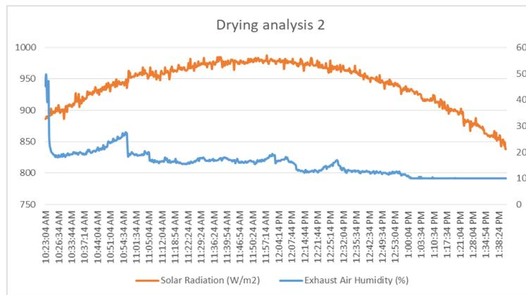
**Figure 6b.** Solar irradiance and humidity during experiment on a high irradiance sunny day.
