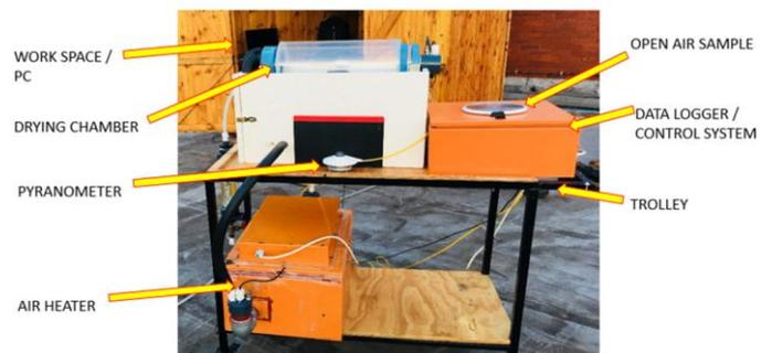
**Figure 2.** Photograph of the solar drying rig
