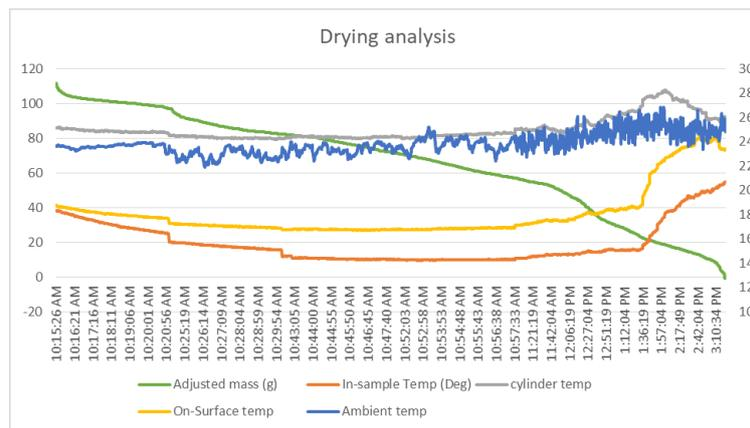
**Figure 7a.** Temperature and mass variations during experiment on a low irradiance sunny day.
