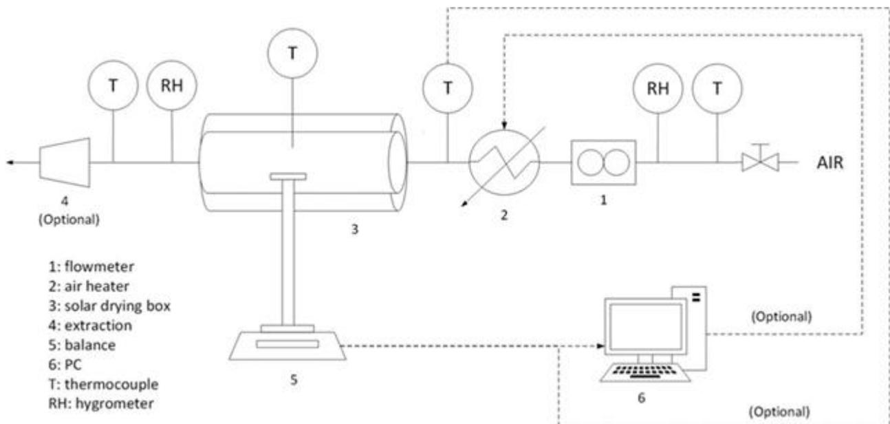
**Figure 3.** Solar drying setup
