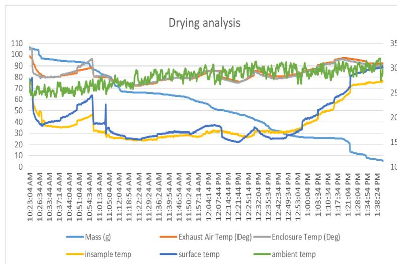
Figure 6a. Temperature and mass variations during experiment on a high irradiance sunny day.
