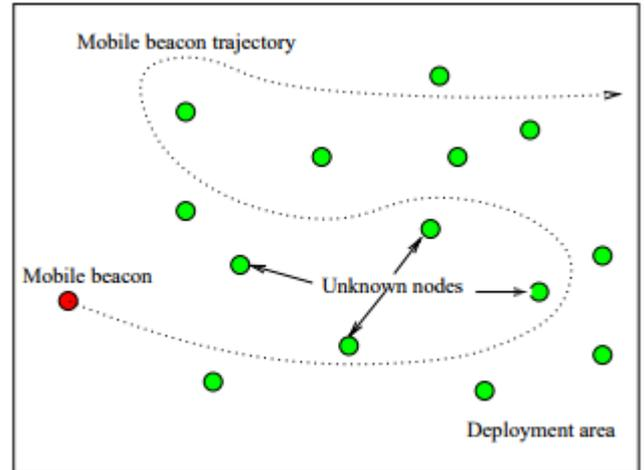
Figure 1. Beacon mobile node assisting for sensor node localization
