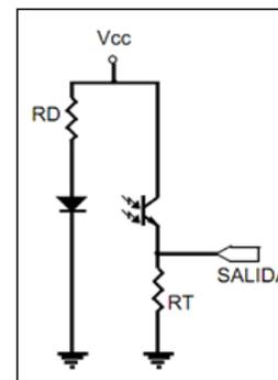
**Figure 8.** Signal adaptation circuit for sensor CNY70
