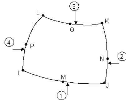
Figure 5: PLANE82 ( 8-node element Structural Solid).
