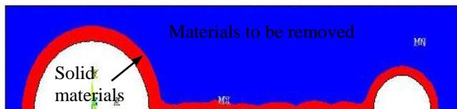
**Figure 9:** The final optimal topological configuration for connecting rod under tension load.
