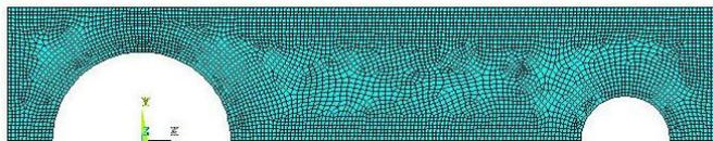
**Figure 7:** Initial two-dimensional mesh for connecting rod.
