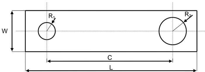
Figure 3: Full model of the connecting rod.
