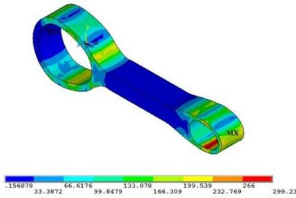
**Figure 14:** von-Mises stress distribution of the three-dimensional optimal topological optimization of connecting rod under tension load.
