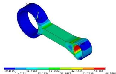
**Figure 13:** von-Mises stress distribution of the three-dimensional optimal topological optimization of connecting rod under compression.
