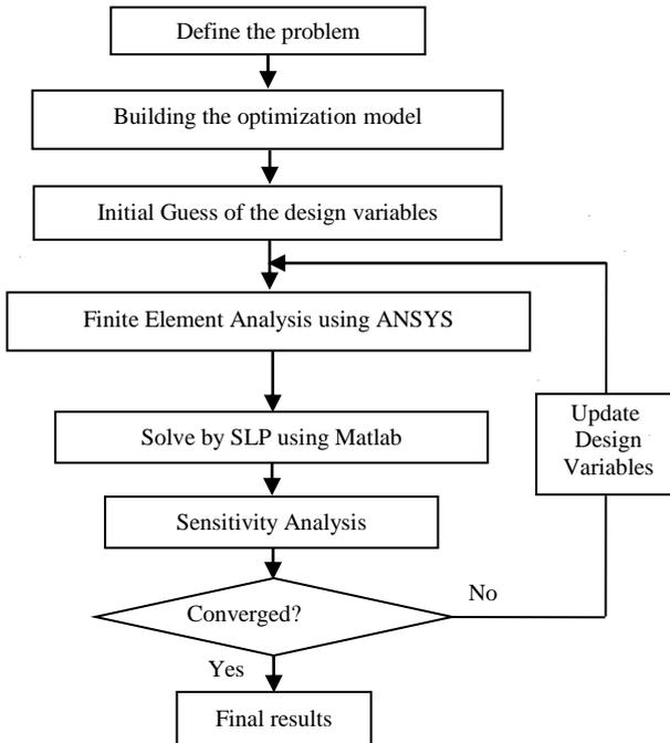
Figure 1: Structural topology optimization flow chart.
