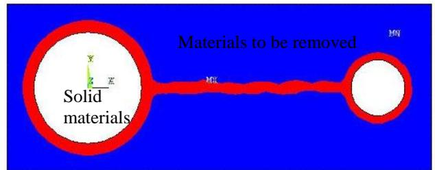
**Figure 11:** The full two-dimensional optimal topological optimization for connecting rod under tension load.
