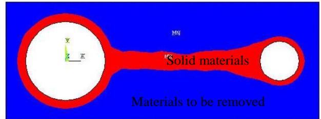
**Figure 10:** The full two-dimensional optimal topological optimization for connecting rod under compression load.
