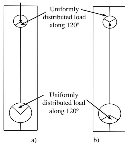
Figure 6: The Loading and boundary conditions: a) compressive load, b) tensile load.
