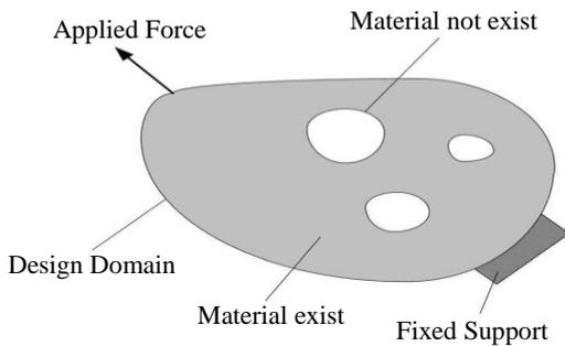
Figure 2: General schematic diagram of the topological structure design.
