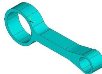
**Figure 12:** the final three dimensional model for the connecting rod.
