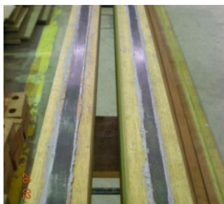
Figure 2. Timber beams strengthened with CFRP plates
