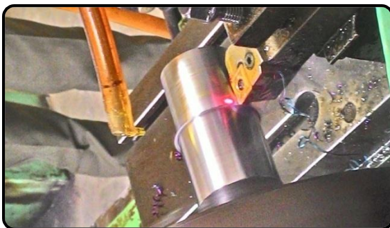
Figure 6. Lubricant dropping on cutting zone
