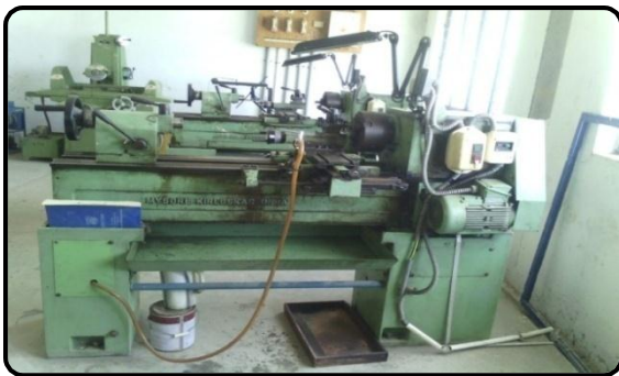
Figure 5. Kirloskar model Turn master 35 centre lathe
