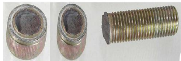
Figure 1. Typical Fastener Failure by Hydrogen Embrittlement [8]
