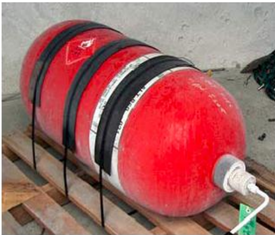
Figure 2. High Pressure Hydrogen storage tank [6]
