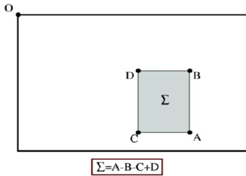
**Figure 2.** Integral Image and its coordinates
