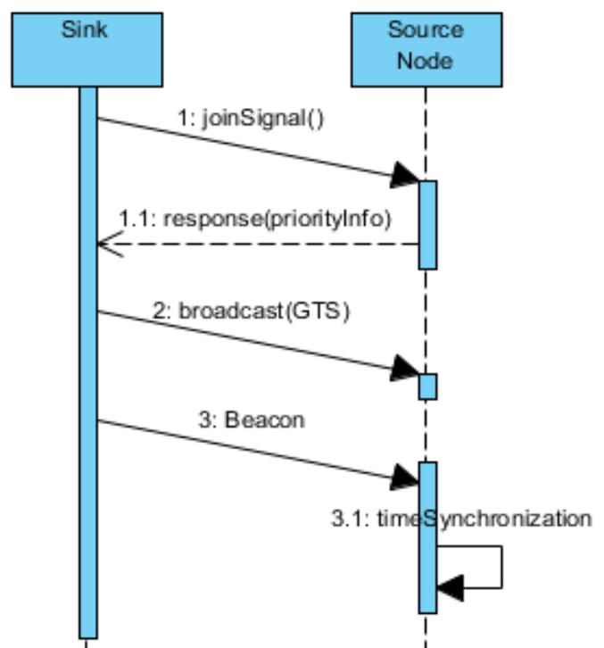
**Figure 1.** shows how the sink node coordinates to the source nodes and gathers priority information for the assignment of GTS slots.
