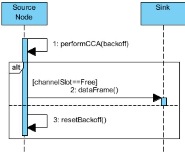
Figure 2(a). Contention-based transmission behavioral view of the no-priority nodes.
