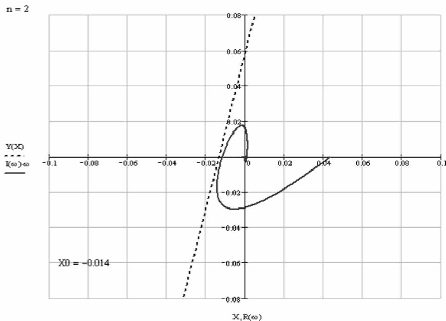
**Figure 5.** Relative position of the hodograph and Popov straight line  $n = 2$ .
