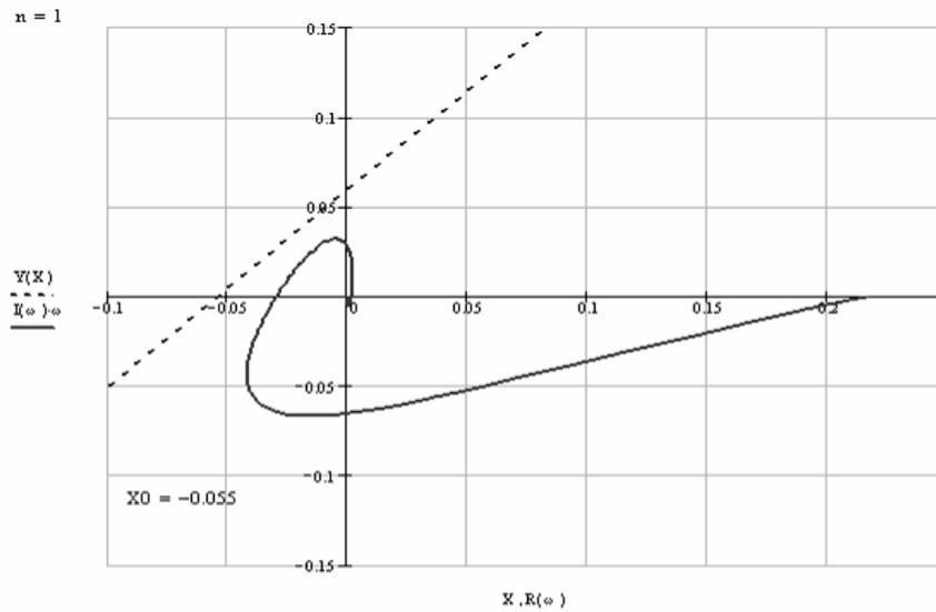
**Figure 4.** Relative position of the hodograph and Popov straight line  $n = 1$ .
