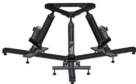
Figure 1. Visualization of the parallel robotic platform imported from the 3D model of the SolidWorks program
