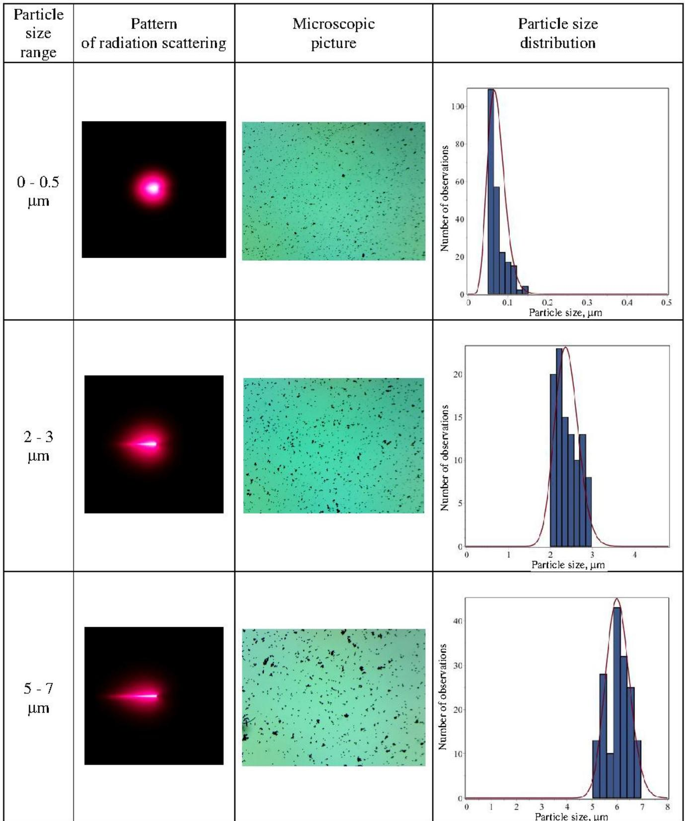
**Figure 3.** Patterns of radiation scattering and the corresponding particle size distributions
