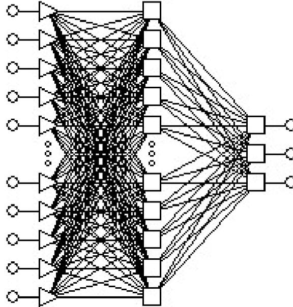
**Figure 5.** The structure of neural network: MLP with the number of neurons in layers 180-25-3
