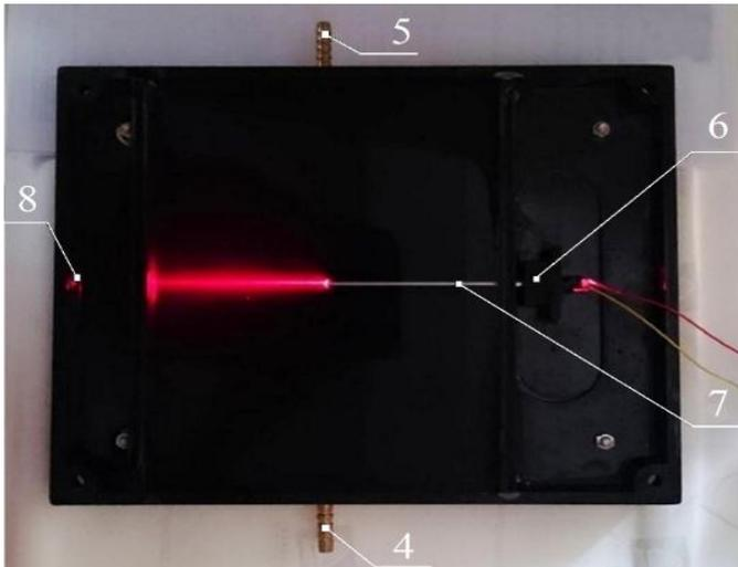
**Figure 2.** The experimental model of the flow measurement chamber
