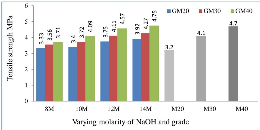
**Figure 3.** Comparison of Splitting tensile strength
