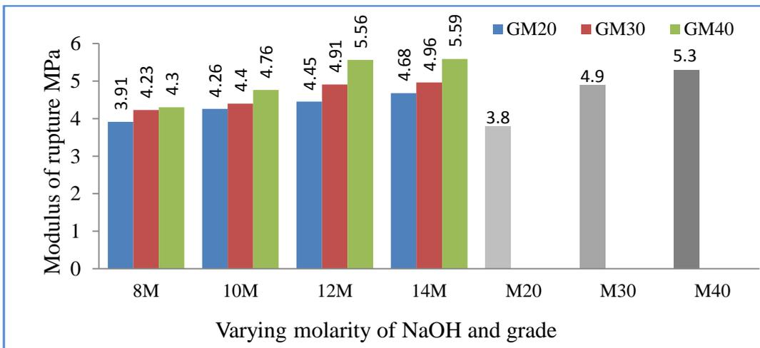
**Figure 4.** Comparison of flexural strength
