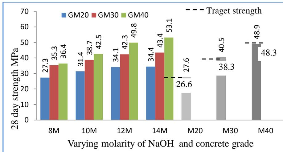
**Figure 2.** Comparison of cube compressive strength
