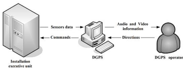
Figure 1: The scheme of the localized interaction between the components and the user of the installation
