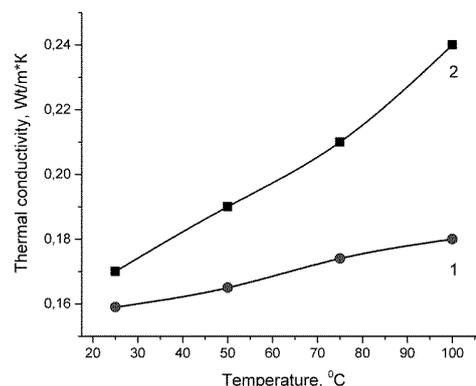
**Figure 2.** Temperature dependence of thin-film HIC with glass (curve 1) and ceramic (curve 2) microspheres (50% of the binder).
