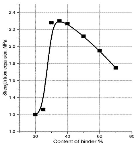
**Figure 6.** Tensile strength of the heat-insulation coating versus the content of polyacrylic binder with hollow glass microspheres.
