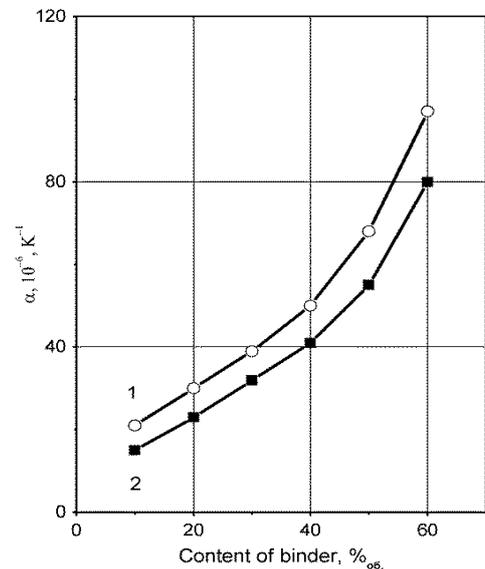
**Figure 4.** The linear thermal expansion coefficient (LTEC) versus content of the binder in thin-film HIC (curve 1 – glass spheres, curve 2 – ceramic spheres).
