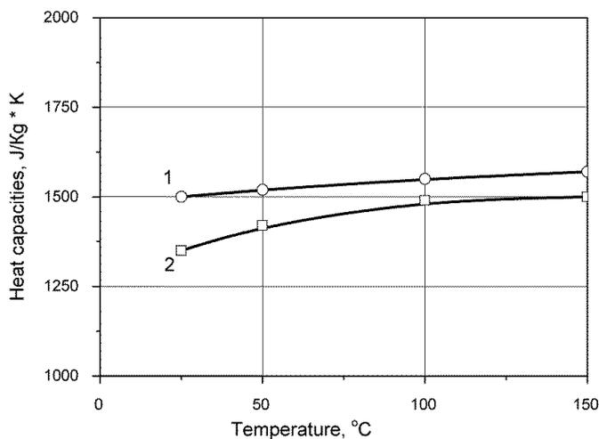
**Figure 3.** Specific heat capacity of the thin-film HIC versus temperature (curve 1 – glass spheres, curve 2 - ceramic spheres)
