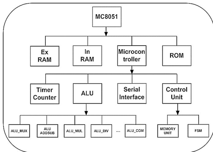
Figure 2: 8051 Block diagram
