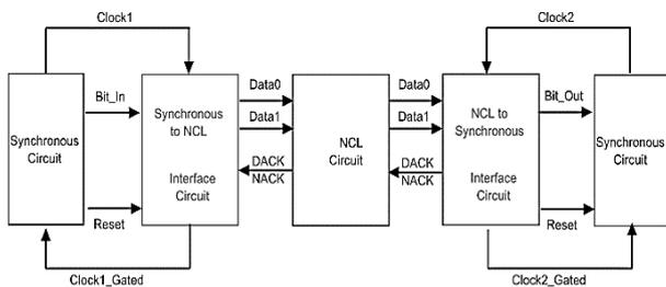
**Figure 5:** Interfacing between synchronous and asynchronous circuits
