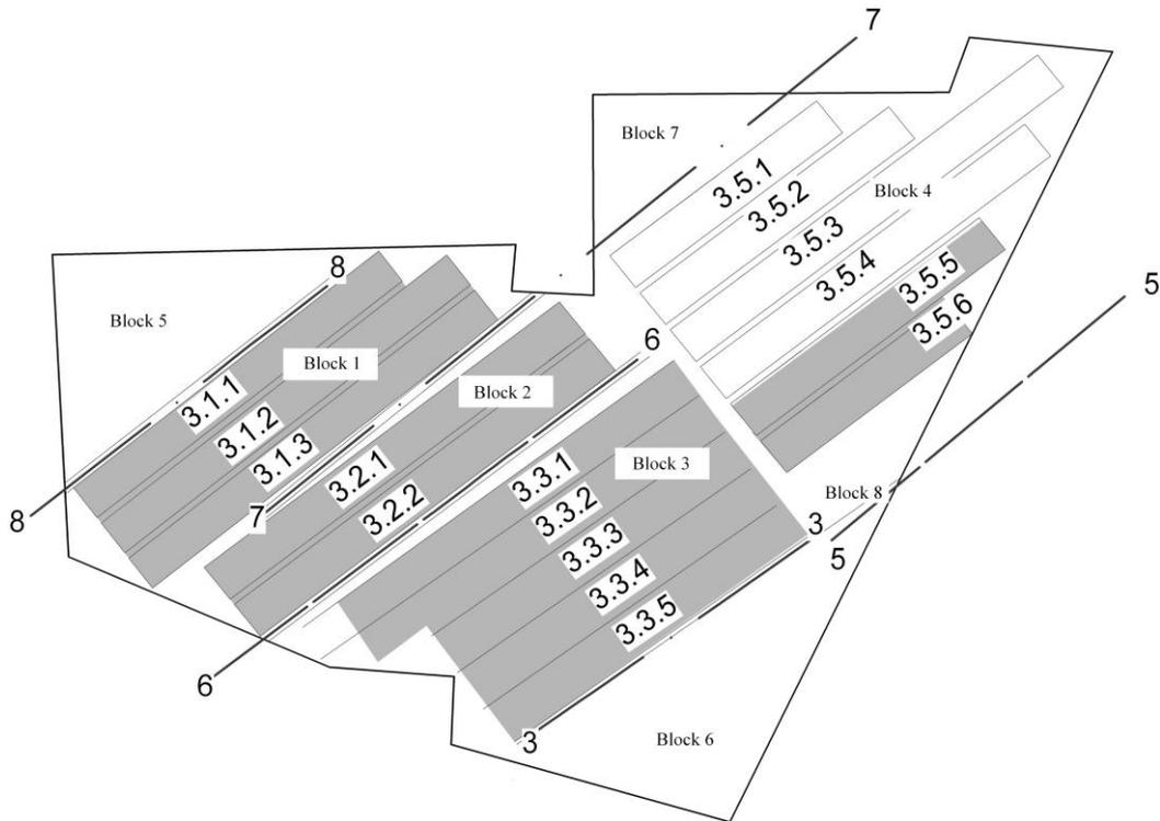
**Figure 3.** Reduced stress zones on the seam III when developing the seam VI using long-pillar system, with the pillars arranged parallel to geological disturbances
