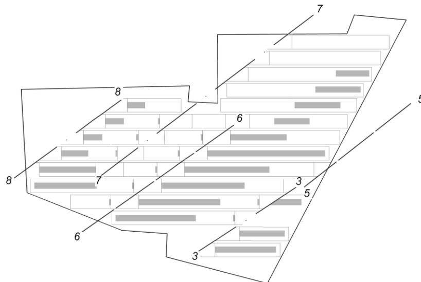
**Figure 2.** Zones of reduced stress on the seam III in case of the seam IV system of mining by long pillars along strike leaving coal pillars between adjacent areas (field No. 2 of the "Raspadskaya-Koksovaya" mine): 8-8, 7-7, 6-6, 3-3, 5-5 – disjunctive geological disturbances
