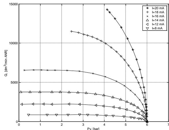
**Figure 2:** Flow-rate curves for  $p_m=6$  bar and different currents  $I$
