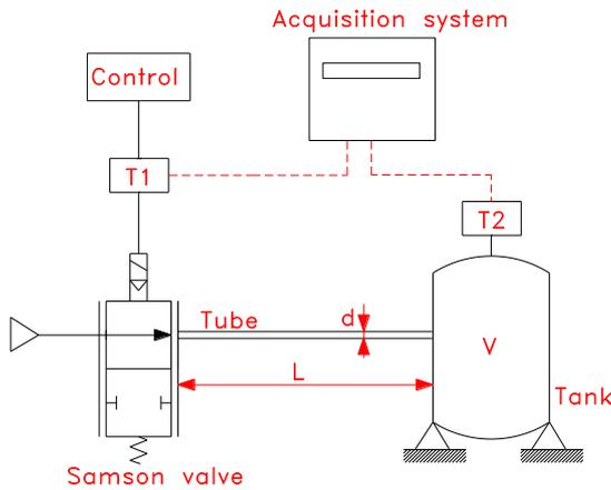
**Figure 7:** Experimental test bench
