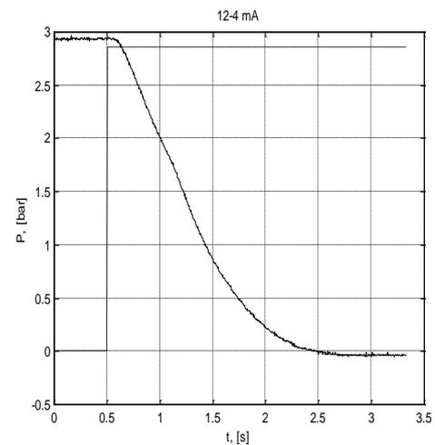
**Figure 6:** Output pressure vs. time for decreasing current  $I$  (12-4 mA) and  $p_m=6\text{ bar}$
