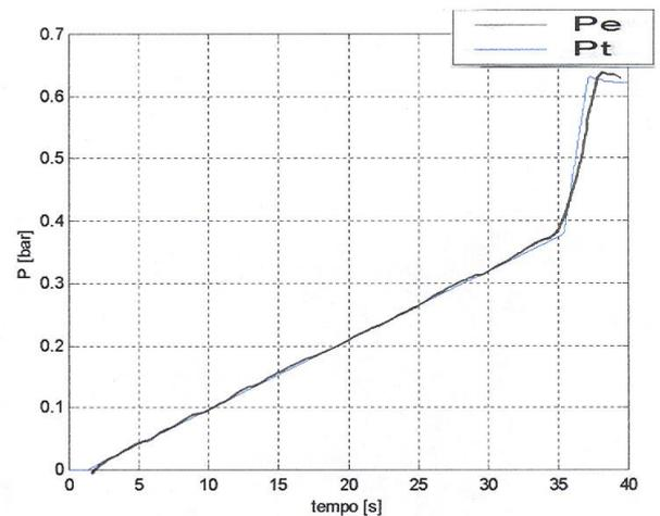
**Figure 9:** Experimental and theoretical pressure inside the furnace
