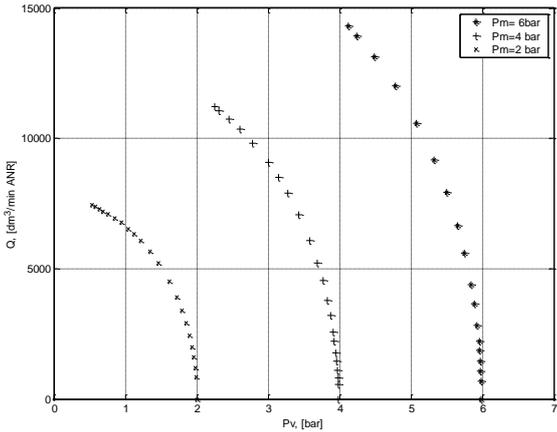
**Figure 3:** Flow-rate curves for  $I=20\text{mA}$  and different  $p_m$
