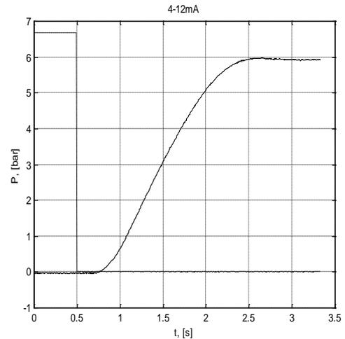
**Figure 5:** Output pressure vs. time for increasing current  $I$  (4-12 mA) and  $p_m=6\text{ bar}$
