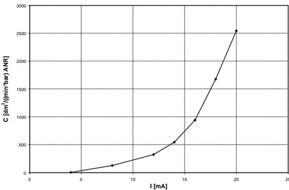
**Figure 4:** Conductance  $C$  vs. pilot current  $I$
