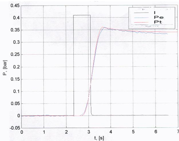
**Figure 8:** Experimental and theoretical pressure inside the tank
