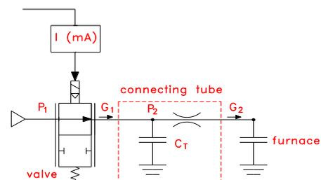
**Figure 1:** Scheme of the low-pressure furnace
