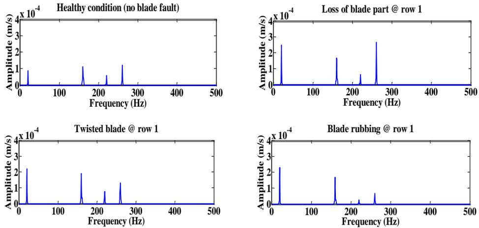
**Figure 5.** FFT spectra for various types of blade fault conditions.
