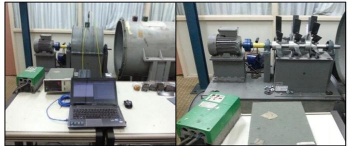
**Figure 2** Multi-stages rotor system and the data acquisition system set up in the experiment
