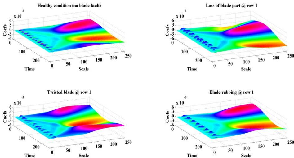
**Figure 6** Wavelet map for various types of blade fault conditions.
