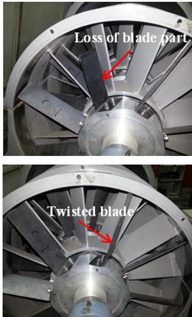
**Figure 3** Type of blade faults
