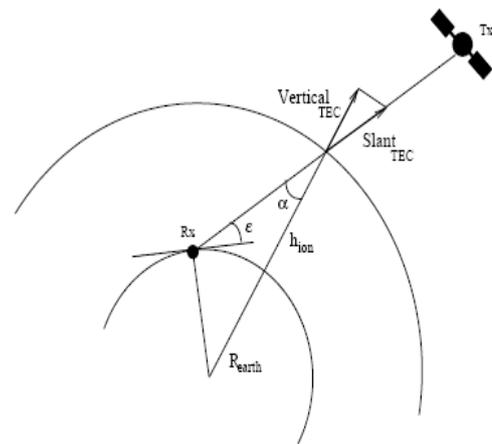
**Figure.1** SLM or thin layer model where TX is transmitter and RX is receiver.
