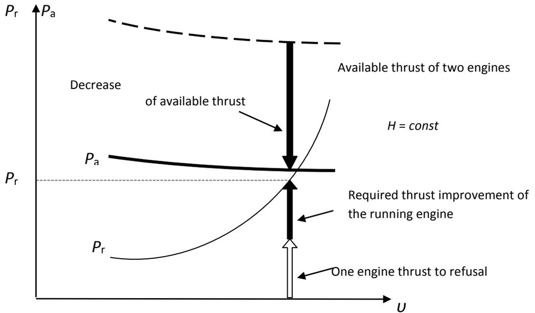
**Figure 5.** Curves of available and required thrust
