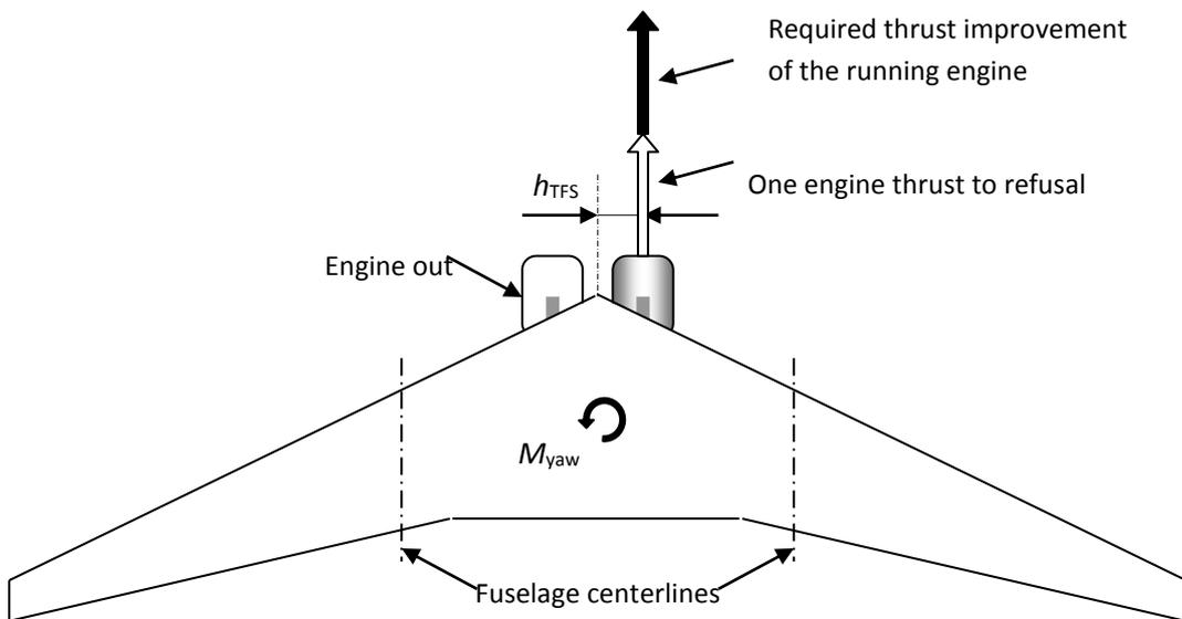
**Figure 6.** Yaw at engine failure
