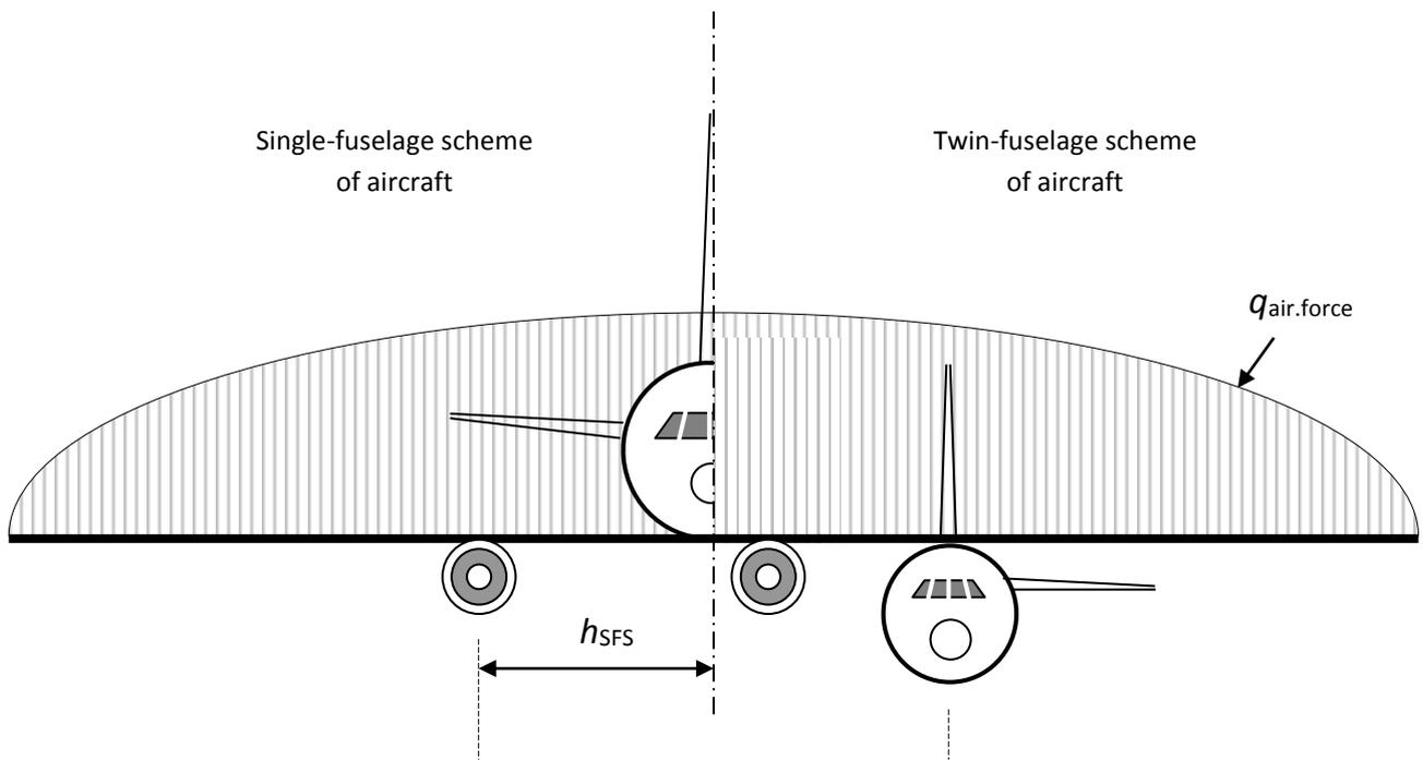
**Figure 3.** Intensity variation of the span-distributed-load
