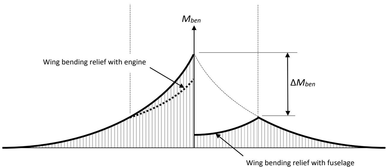
**Figure 4.** The bending-moments curve
