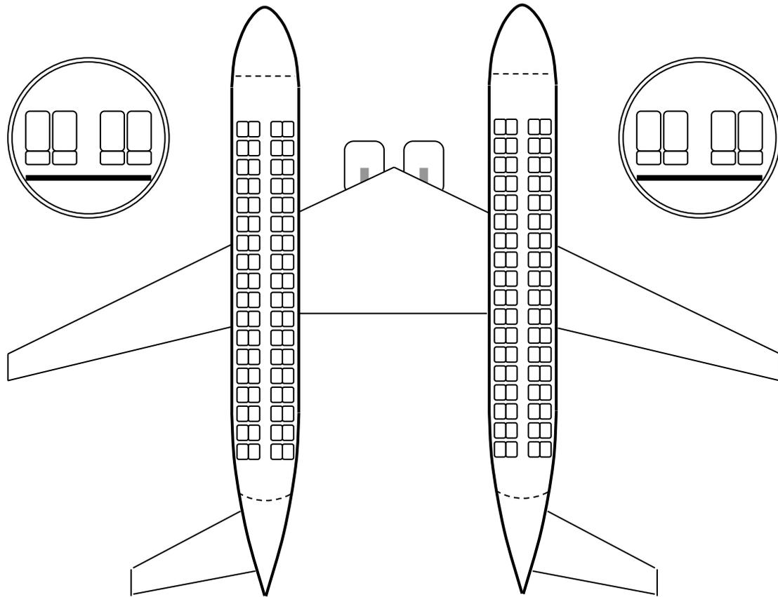
**Figure 2.** The configuration of the medium-haul twin-fuselage passenger aircraft
