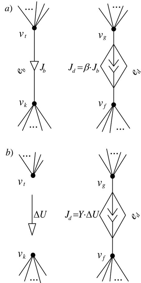
Figure 2: Controlled current sources: a – CCCS; b – VCCS
