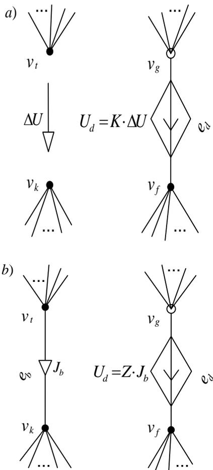
Figure 1: Controlled voltage sources: a – VCVS; b – CCVC
