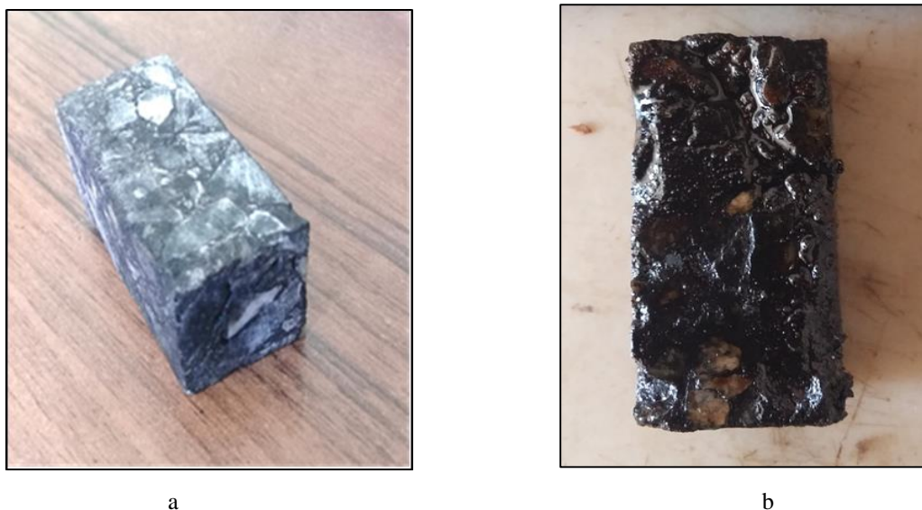
Figure 4: Rectangular bitumen core samples (a) before experiment, (b) after experiment
