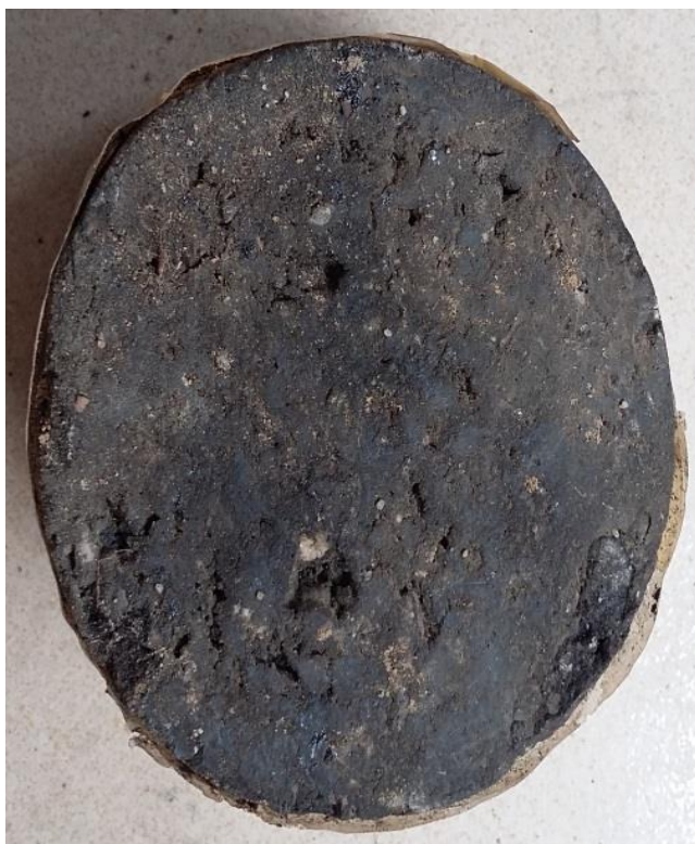
Figure 3: Cylindrical bitumen core sample from Yegbata Well 1, before cutting into rectangular shapes
