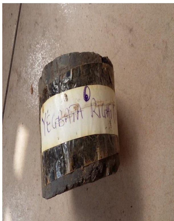
Figure 3: Cylindrical bitumen core sample from Yegbata Well 1, before cutting into rectangular shapes
