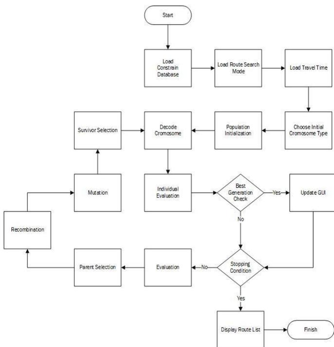
**Figure 2:** Genetic Algorithm Work Flow System [1]
