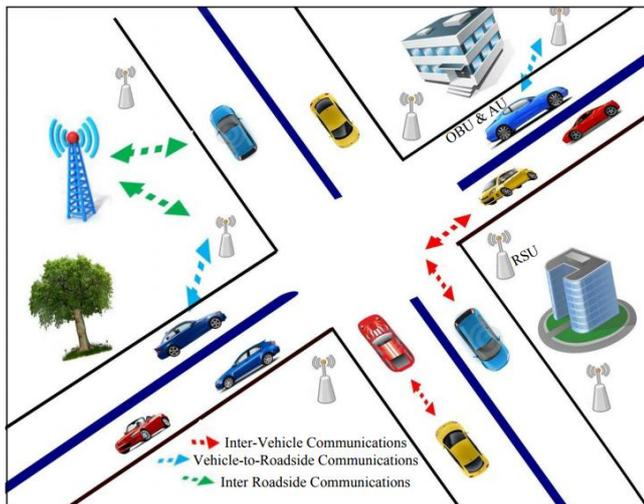
**Figure 4:** A typical VANET Scenario Using Ant Colony Algorithm [12]
