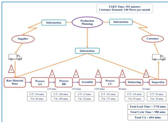
**Figure 3:** Current state value stream mapping
