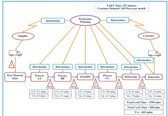
**Figure 4:** Future state value stream mapping
