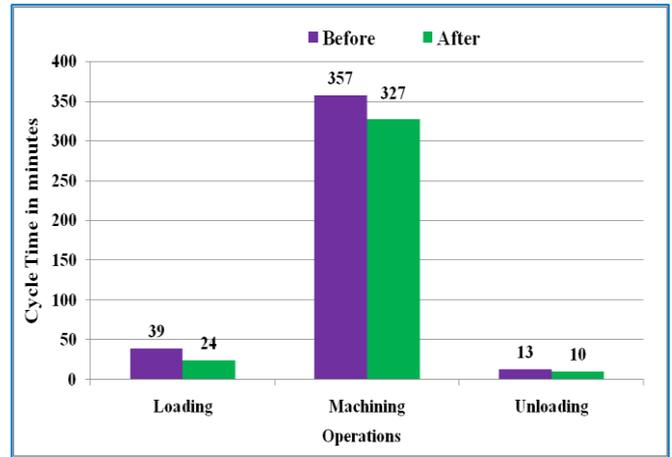
**Figure 13:** FTF cycle time for process CC
