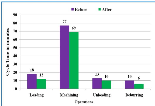
**Figure 11:** FTF cycle time for process AA
