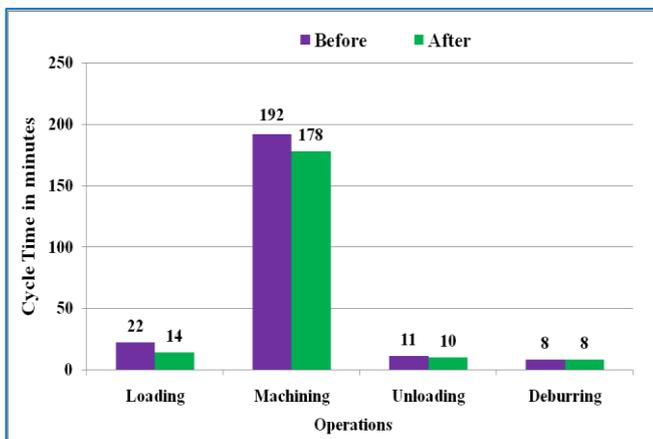
**Figure 12:** FTF cycle time for process BB
