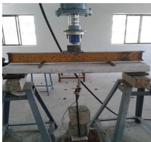
Figure 4: Loading setup of slab specimen.
