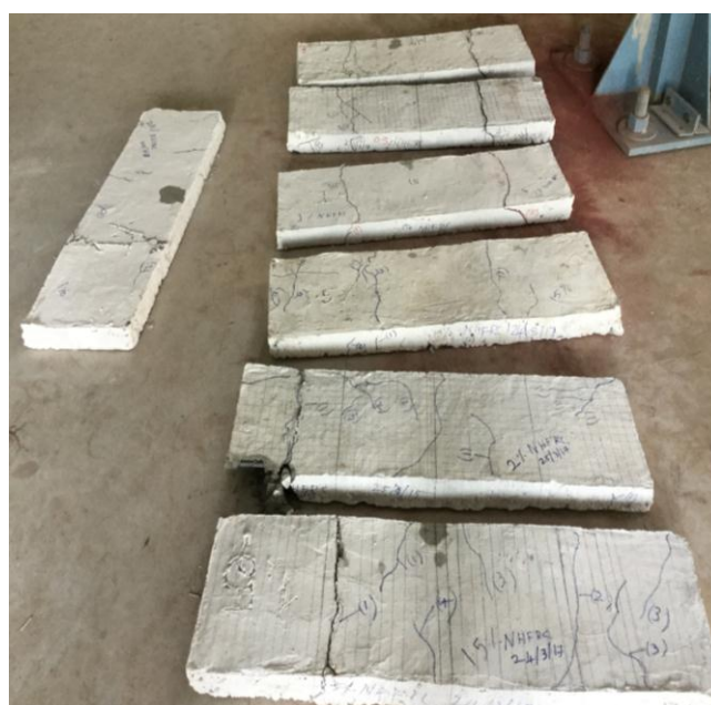
Figure 6: Slab specimen after failure of various percentages
