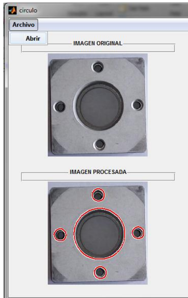
Figure 3: GUI designed in MATLAB with displayed circle detection
