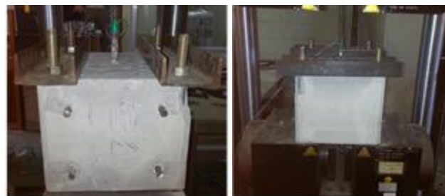
(b) Pullout strength experimental setup
