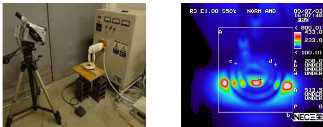
Figure 3: Thermography and measured heat image screen
