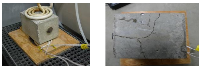
Figure 10: Sample of a test body after it is heated and cracks are induced
