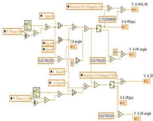
**Figure 10:** (c) Voltage calculation for one of the phase (A) on HV and LV sides of transformer
