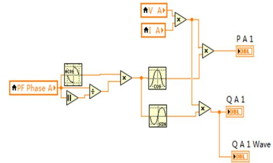
**Figure 10:** (d) Active and Reactive Power calculation after compensation
