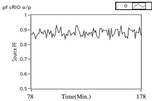
Figure 6: (b) p.f. for one phase as monitored by cRIO
