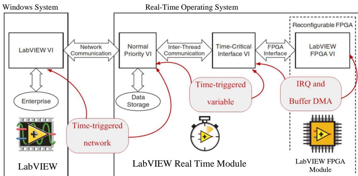
**Figure 3:** LabVIEW FPGA Architecture for Real-Time [11]
