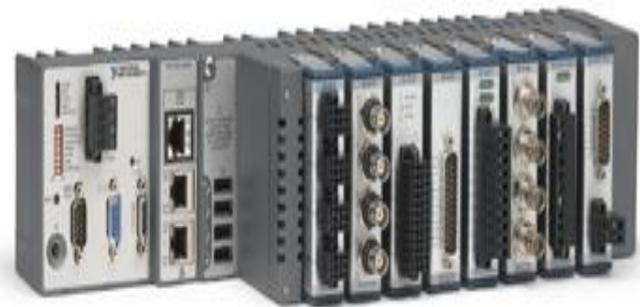
**Figure 4:** (b) NI cRIO-9082 chassis with all the I/O modules [10]
