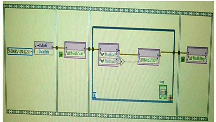
Figure 9: The data acquisition program on LabVIEW FPGA
