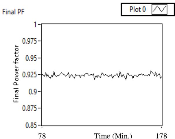
**Figure 12:** (b) Compensated p.f. for one phase
