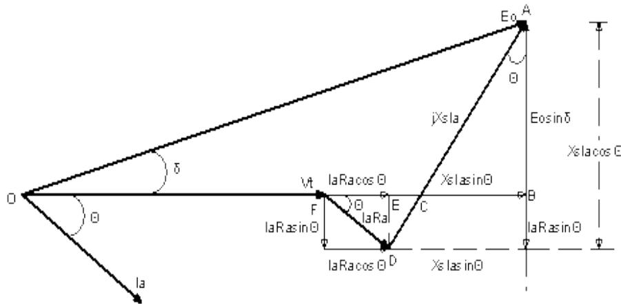
**Figure 1:** Power angle diagram
