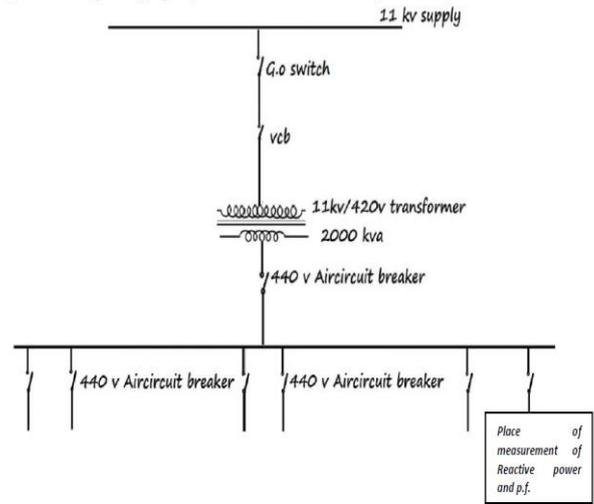
**Figure 5:** Single Line Diagram of 11kV/420V Distribution Transformer Bay
