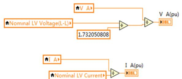
Figure 10: (b) Acquired data conversion to per unit values
