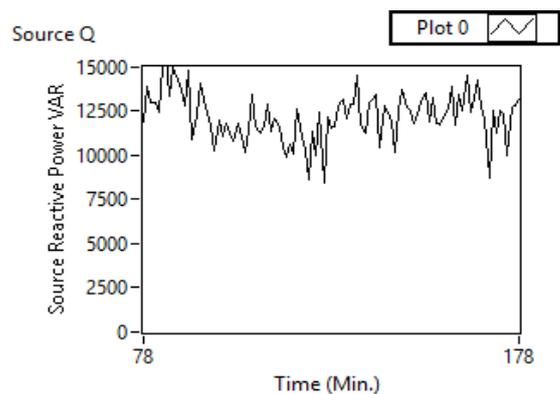
**Figure 6:** (a) Reactive power (in VAR) for one phase as monitored by cRIO
