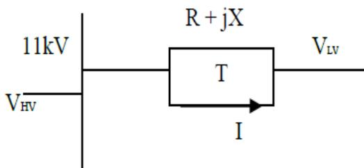
Figure 8: The Transformer model for a single phase.
