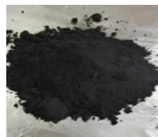
Figure 5. Activated carbon after physical activation process
