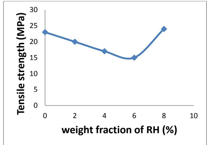
**Figure (3):** The effect of rice husk (RH) weight fraction on tensile strength.
