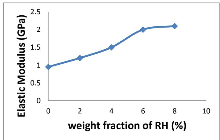
**Figure (4):** The effect of rice husk (RH) weight fraction on elastic modulus.
