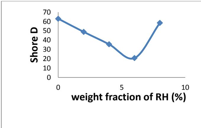
**Figure (1):** The effect of rice husk (RH) weight fraction on the shore D hardness.
