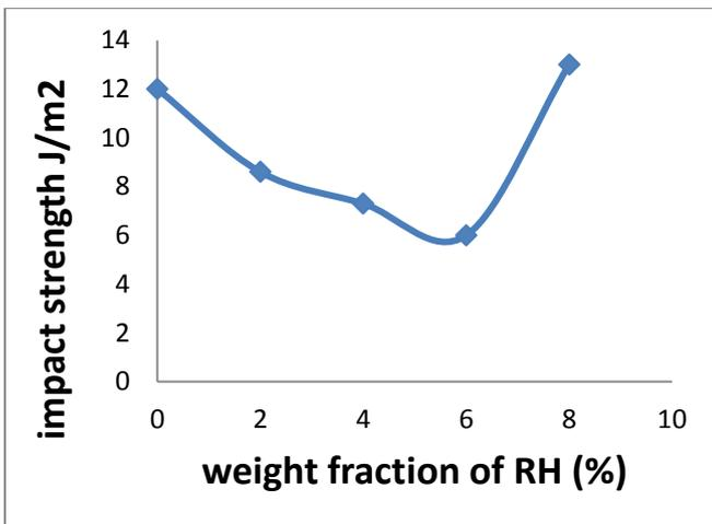
**Figure (2):** The effect of rice husk (RH) weight fraction on impact strength.
