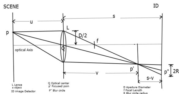
Figure 1: image generation in a convex lens
