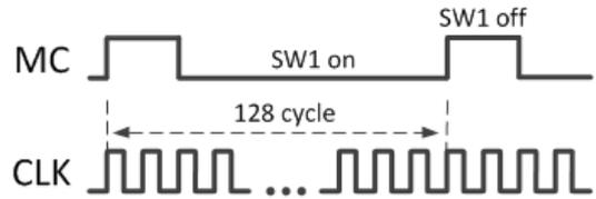
Figure 5: Timing diagram of MPPT clock MC.
