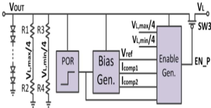
Figure 8: Block diagram of PMU.
