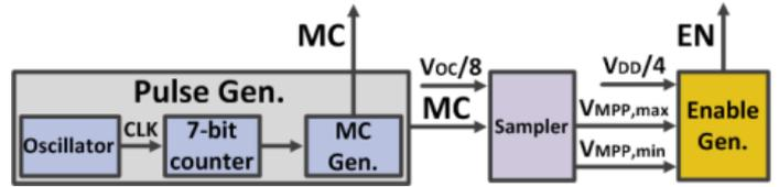
Figure 4: Block diagram of MPPT controller.
