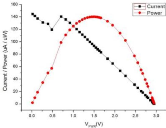
Figure 3: P-V & I-V characteristics of PZT with ADC.
