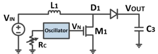
Figure 6: DC-DC boost converter.
