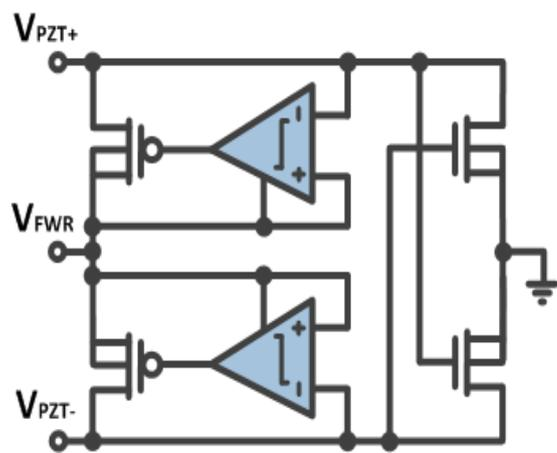
**Figure 2:** AC-DC converter (ADC).
