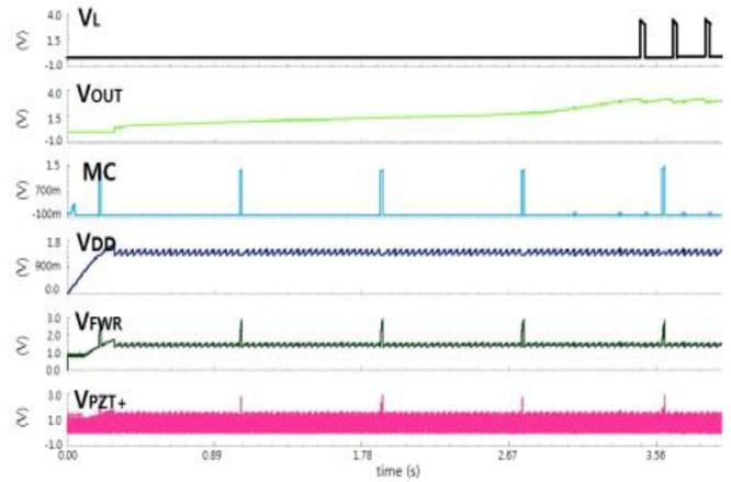
Figure 10: Simulation results of the entire circuit.
