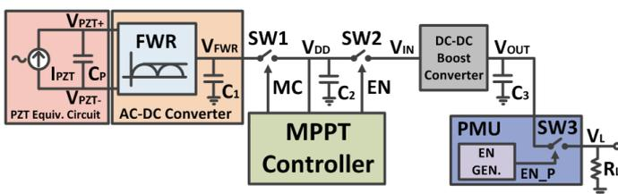
**Figure 1:** Block diagram of the proposed vibrational energy harvesting circuit.
