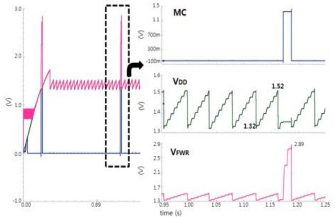
Figure 11: Magnified waveforms of the start-up transient and MPPT control.
