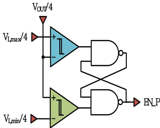
Figure 9: Enable generator.
