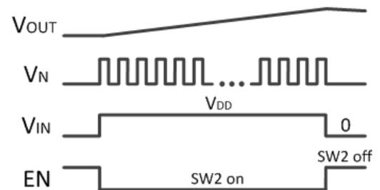
Figure 7: Operation waveforms of DC-DC boost converter.
