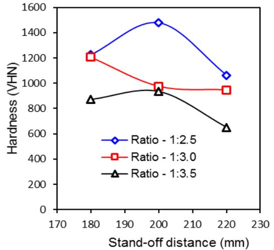
**Figure 4:** Parametric influence on hardness
