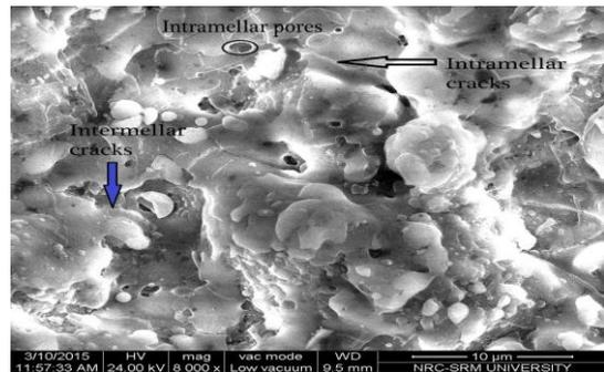
(a) Standoff - 180mm, Coating thickness - 200 µm
