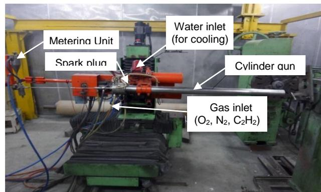
**Figure 1:** D-gun coating set-up
