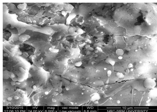
Fig. 8 (a) Standoff -180 mm, Coating thickness - 200 μm
