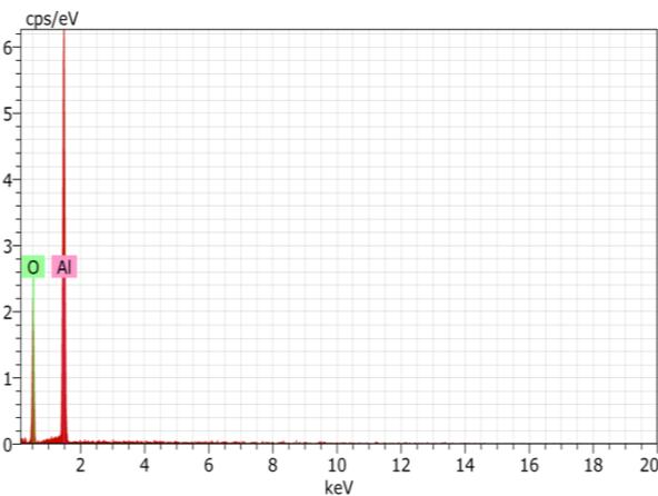
**Figure 3:** EDS Analysis of Alumina powder sample
