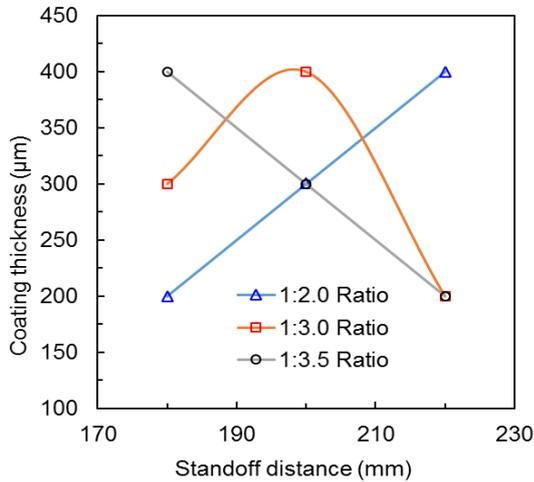
Figure 6: Parametric influence on coating thickness
