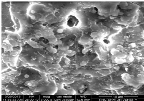
(a) Standoff - 80 mm, Coating thickness - 300 μm
