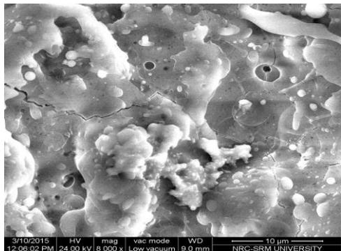
Fig. 8 (c) Standoff - 220 mm, Coating thickness - 200  $\mu\text{m}$
