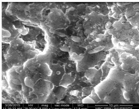
(b) Standoff – 200 mm, Coating thickness – 400 μm
