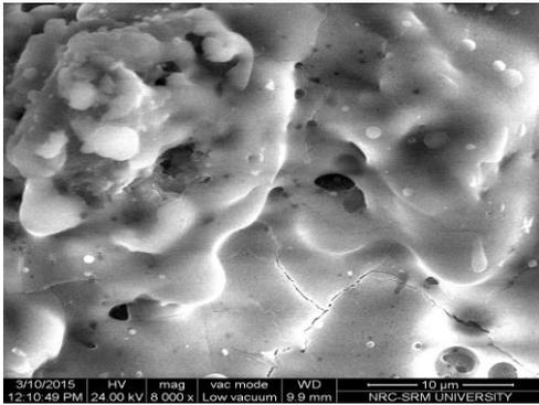
Fig. 8 (b) Standoff - 200 mm, Coating thickness - 300  $\mu\text{m}$
