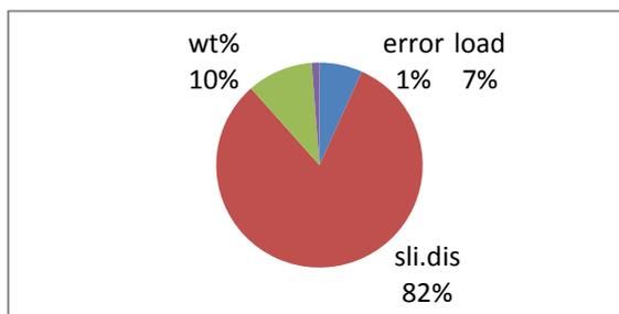
**Figure 7:** contribution of the process parameter on the wear rate
