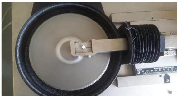
**Figure. 4:** View of wear testing tribometer (DUCOM)
