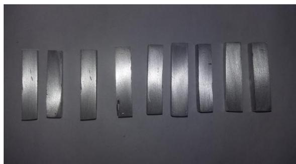
**Figure 3:** Pin type samples for wear testing
