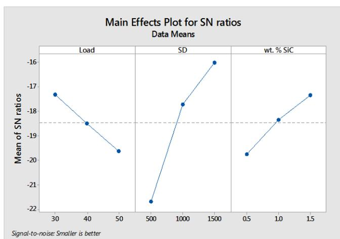
**Figure. 5:** Main effects plot for S/N ratios (wear rate)
