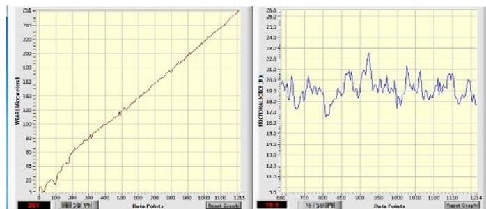
**Figure 2:** Showing wear (in micrometer) and frictional force w.r.t time (seconds)
