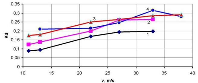
**Figure 5:** Comparison of calculated and experimental mean square values of the coefficient of dynamics of the second stage of suspension
