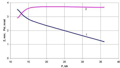
**Figure 4:** Amplitudes of forced body oscillations in dependence on the magnitude of the dry friction force in the suspension of the body
