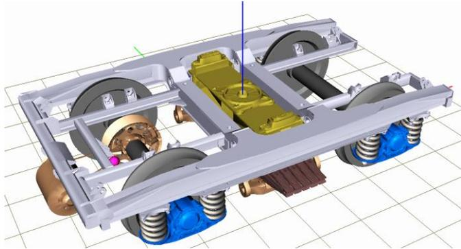
**Figure 1:** Model of the KVZ-I2 bogie in the "Universal Mechanism" software package
