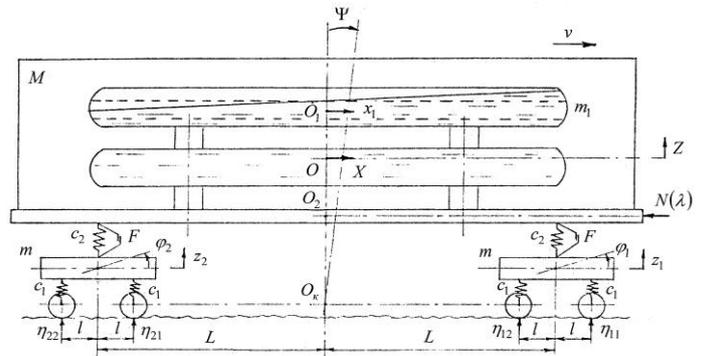
**Figure 2:** Calculation scheme of the cryogenic section
