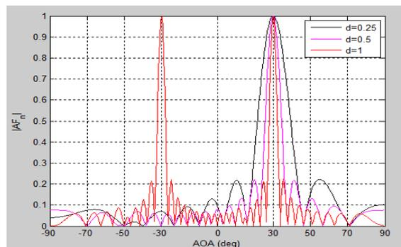
**Figure 3.c:** Effect of interelement spacing on Array Factor.
