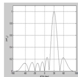
**Figure 4.c):** Array Factor versus Angle of Arrival when desired signal is at 0dB and interferer signal is at 5dB
