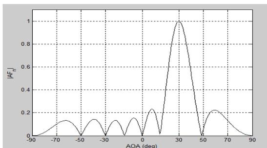
**Figure 1.b:** Array factor plot when desired user is 30° and the interferer is -50°
