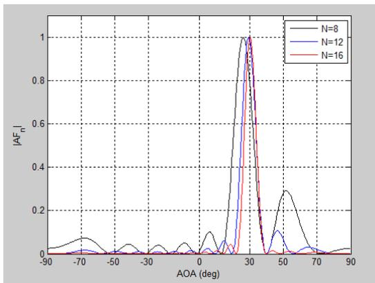
**Figure 6.d):** array factor plot when desired user is 30°, and interference is 40°, for N=8, 12 and 16
