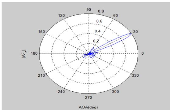
**Figure 1.a:** Polar array factor plot when desired user is 30° and the interferer is -50°
