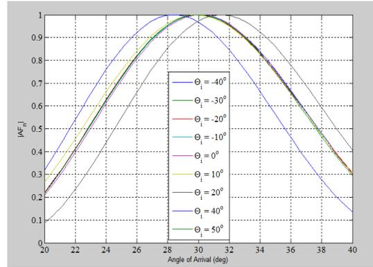
**Figure 6 b):** Array Factor versus Direction of Arrival when desired angle is at 30° for different interferences: -40°, -30°, -20°, -10°, 0°, 10°, 20°, 40°, and 50° (with x axis zoomed)
