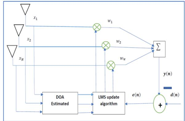
**Figure. 3.1:** LMS adaptive Array System
