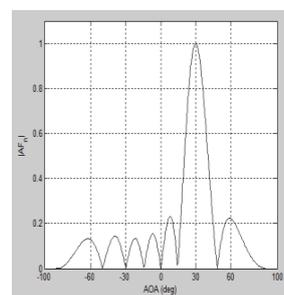
**Figure 4.a):** Array Factor versus Direction of Arrival when desired signal is at 0dB and interferer signal is at 0dB
